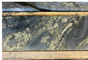
Right photo: chalcopryite-pyrite stringers in intensely chlorite-sericite alteration of the host felsic volcanic rocks.
